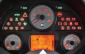
**The Advanced Dashboard** displays Engine and PTO speeds, service intervals, fuel consumption, distance travelled, area worked, oil temperature and tractor hours, Engine speed memorised, Service information.
