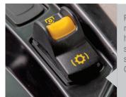
PTO engagement remains electrohydraulic using the same 3-position safety switch (On, Off and Lock/brake).
