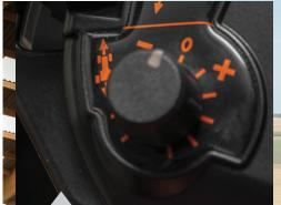
**Comfort Control roller switch** PowerControl lever option : Shuttle responsiveness can be adjusted according to speed of change required to really match the handling job in hand
